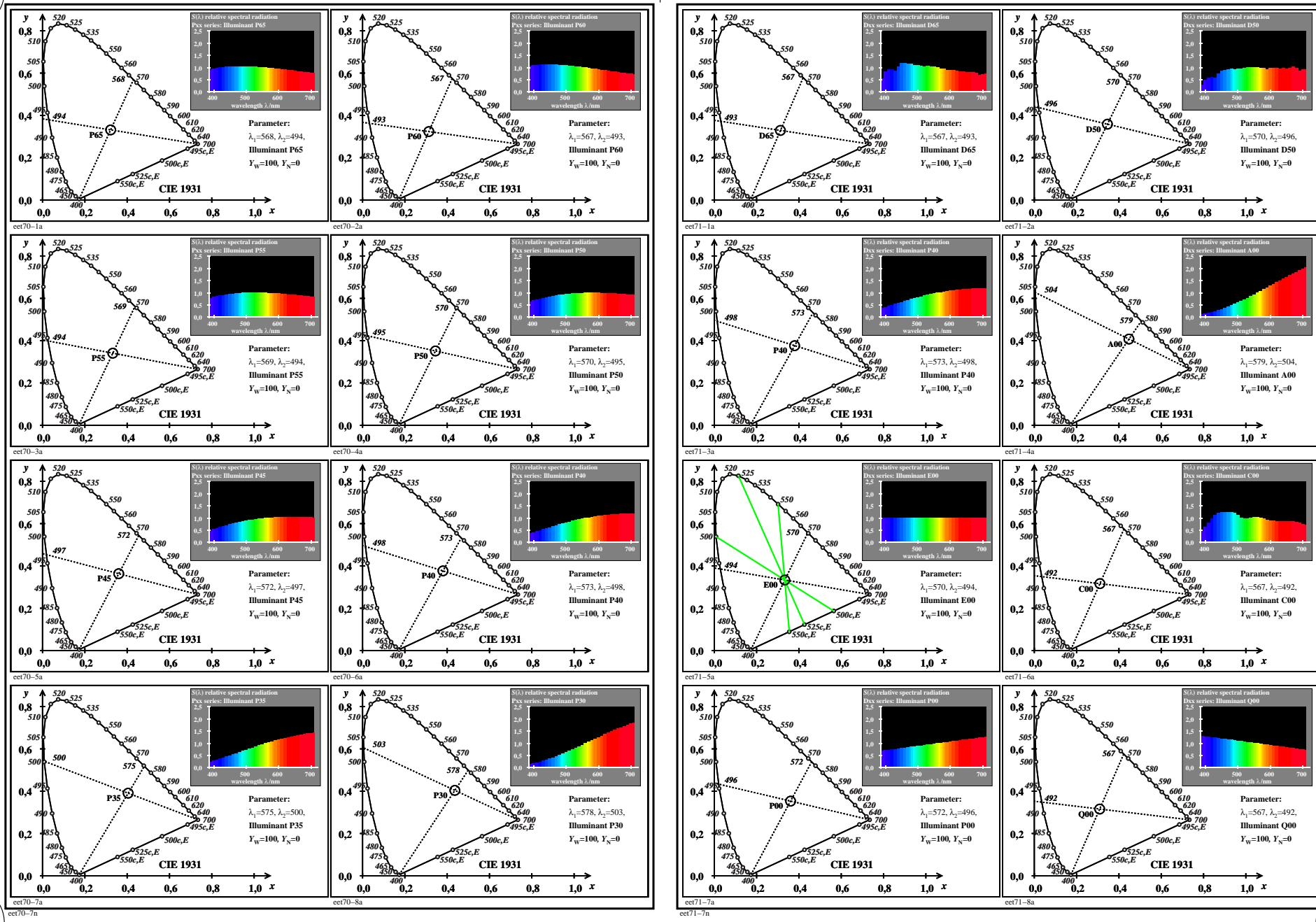
TUB-test chart eet7; 6 Ostwald optimal colours for 8 illuminants Pxx (left) and Dxx (right)
