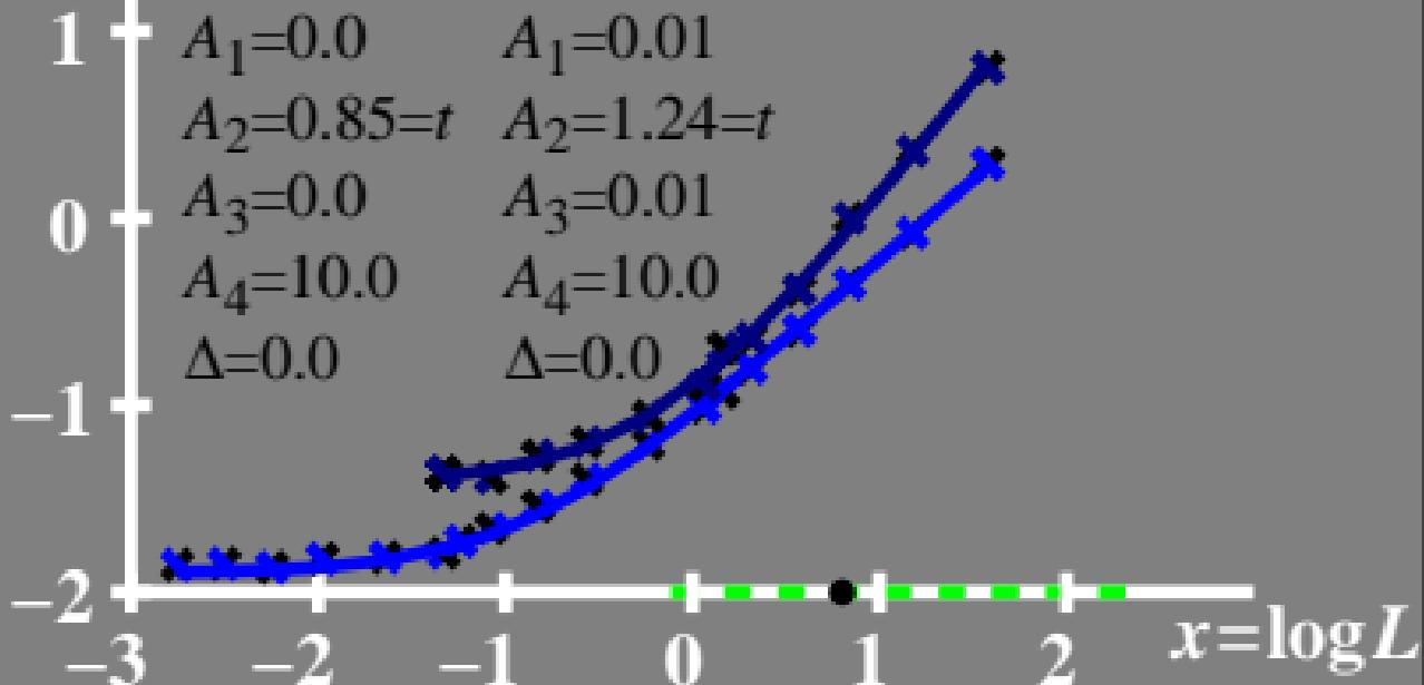
$\log(L/\Delta L)$  luminance contrast sensitivity threshold •  $L_g = 6.3 \text{ cd/m}^2$
