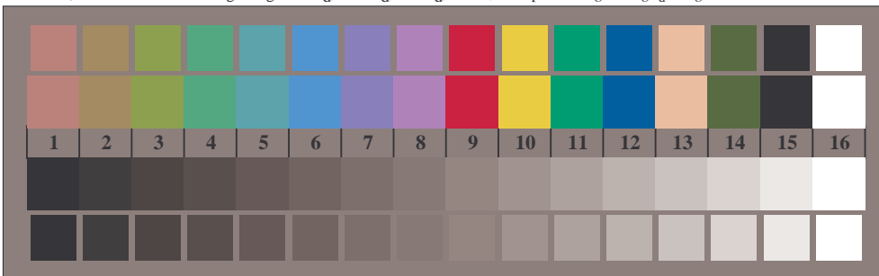
TN980-7, Picture B3Wd: 14 CIE-test colours and 2 + 16 grey steps (sf); PS operator: rgb/cmy0 \rightarrow rgb_d setrgbcolor
