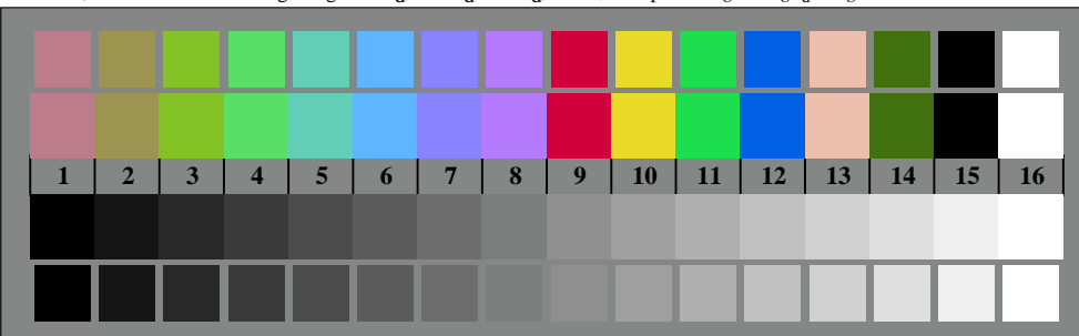
TN810-7, Picture D3Wd: 14 CIE-test colours and 2 + 16 grey steps (sf); rgb/cmy0 \rightarrow rgb_d setrgbcolor
