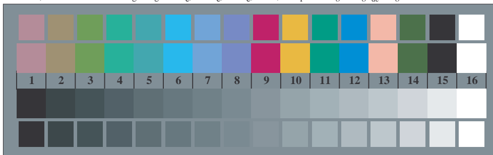
TE880-7, Picture D3Wde: 14 CIE-test colours and 2 + 16 grey steps (sf); PS operator: rgb/cmy0 \rightarrow rgb_{de} setrgbcolor
