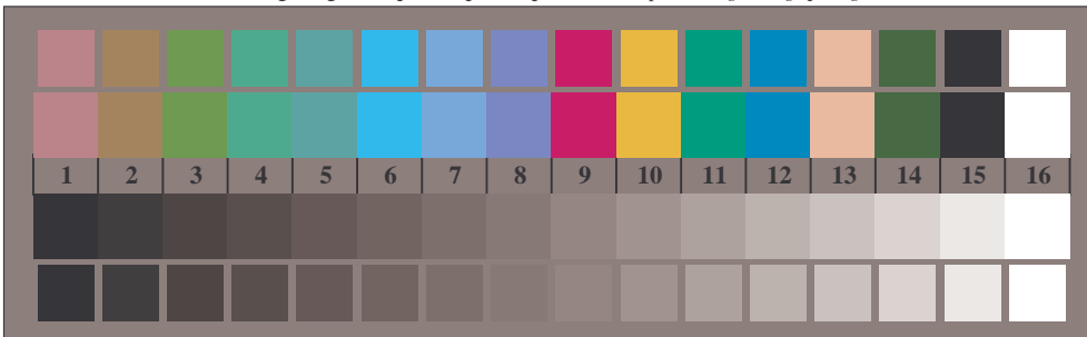
TE880-7, Picture D3We: 14 CIE-test colours and 2 + 16 grey steps (sf); PS operator: rgb/cmy0 \rightarrow rgb_e setrgbcolor
