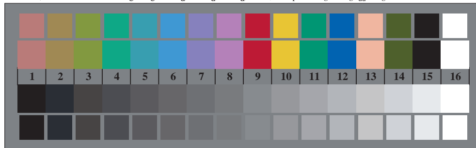
TE840-7, Picture D3Wdd: 14 CIE-test colours and 2 + 16 grey steps (sD); rgb/cmy_0 \rightarrow rgb_{dd} setrgbcolor
