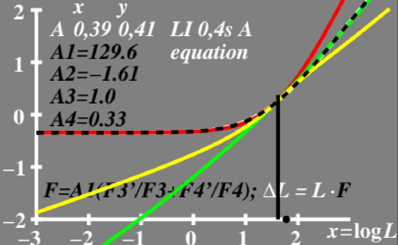
$\log \Delta L$  luminance difference threshold;  $\Delta L = L \cdot F$  •  $L_g = 600 \text{ cd/m}^2$
