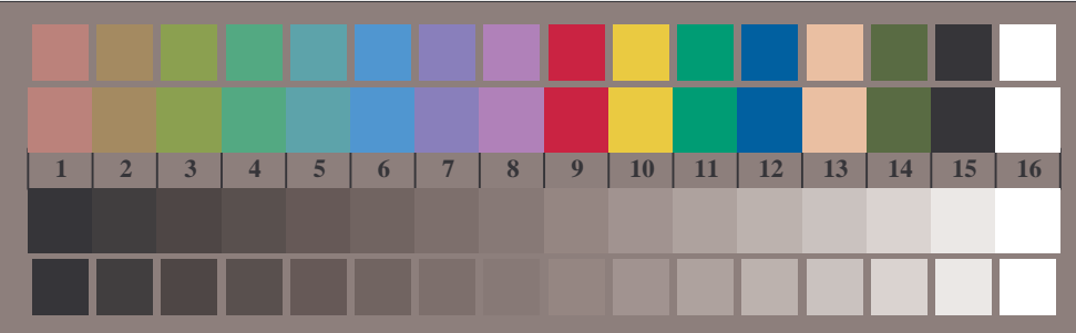
IE800-7, Picture B3: 14 CIE-test colours and 2 + 16 grey steps; Use of PS operator olv* setrgbcolor
