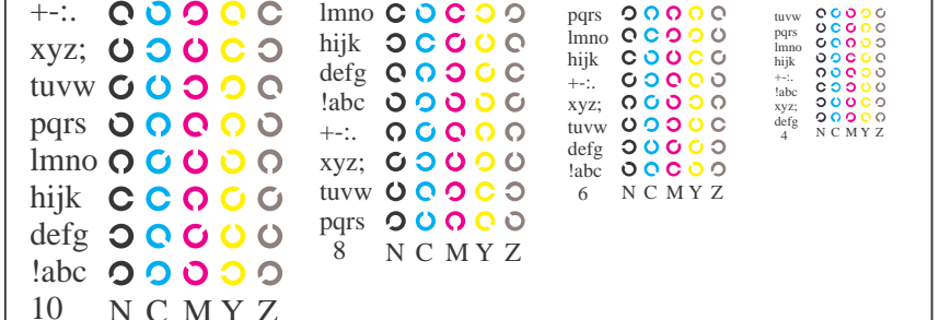
IE801-3, Picture B5: Script and Landolt-rings N, C, M, Y, Z; PS operator olv* setrgbcolor
