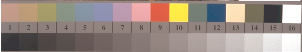
IE800-3, Picture B1: Flower motif, 14 CIE-test colours, 16 grey steps (sf); PS operators settransfer , 4 colorimage
