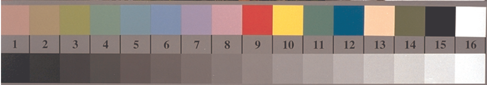
Picture B1: Flower motif, 14 CIE-test colours and 2 + 16 grey steps (nf); PS operators settransfer , 4 colorimage
