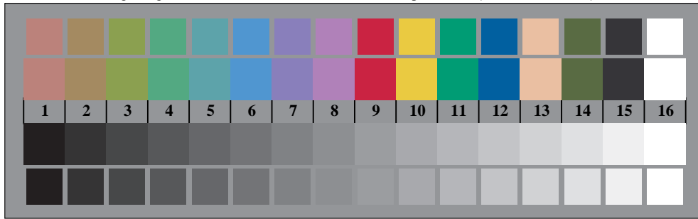
Picture B3: 14 CIE-test colours and 2 + 16 grey steps (sf); PS operator: cmY0*/000n* setcmYcolor
