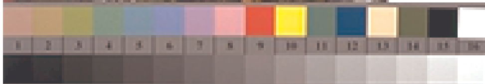
Picture B1: Flower motif, 14 CIE-test colours and 2 + 16 grey steps (sf); PS operators settransfer , 4 colorimage
