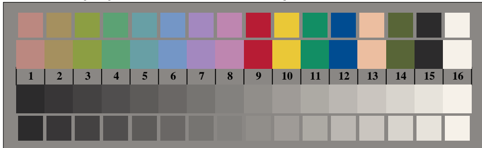
Picture B3: 14 CIE-test colours and 2 + 16 grey steps (sf); PS operator: LAB* setcolor
