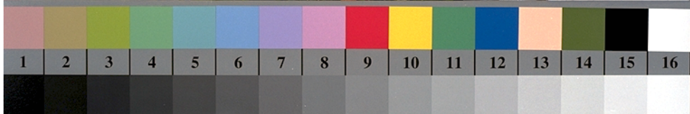
AE280-3, Picture B1Wdd: Flower motif, 14 CIE-test colours and 2 + 16 grey steps (nf); PS operators settransfer , 3 colorimage
