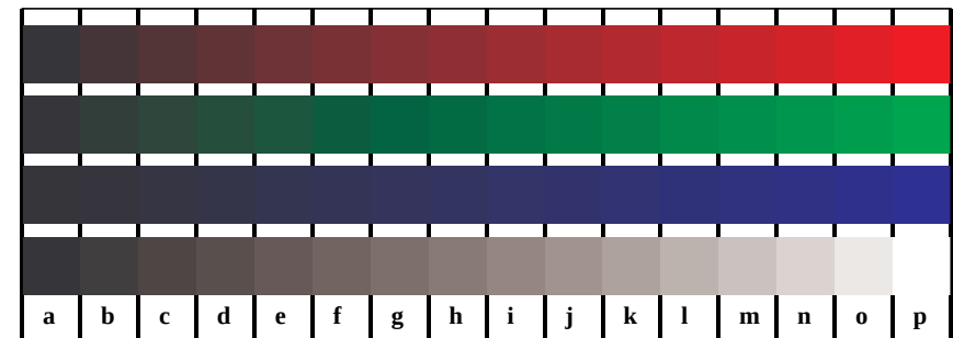
Picture D4n: 16 equidistant steps N-O , N-L , N-V and N-W ; PS operator cmy0* setcmykcolor (only)
