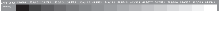
Picture C3: 16 visual equidistant L^* -grey steps; PS operator: 000n*lin 1.0 exp setcmykcolor; use file www.bam.de/KE86/10B/B86E00FA.PS or /B86E00FP.PS for DPS or PDF systems to complete the figure
