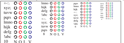
Picture D5: Script and Landolt-rings N, O, L and V; Use of PS operator olv* setrgbcolor (only)
