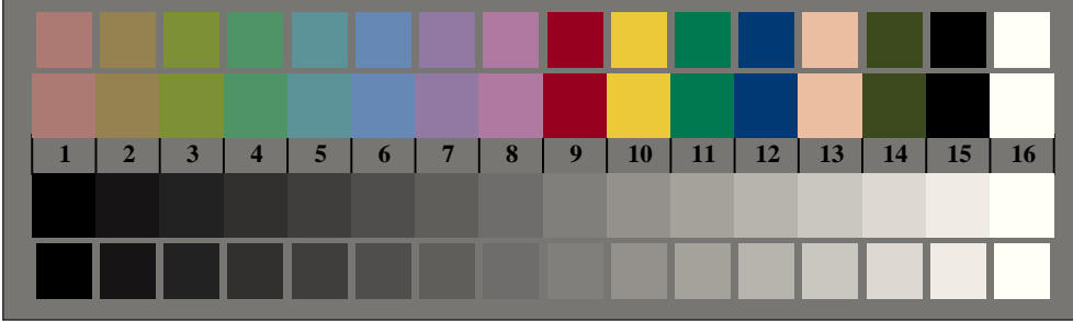
Picture D3: 14 CIE-test colours and 2 + 16 grey steps; Use of PS operator olv* setrgbcolor (only)
