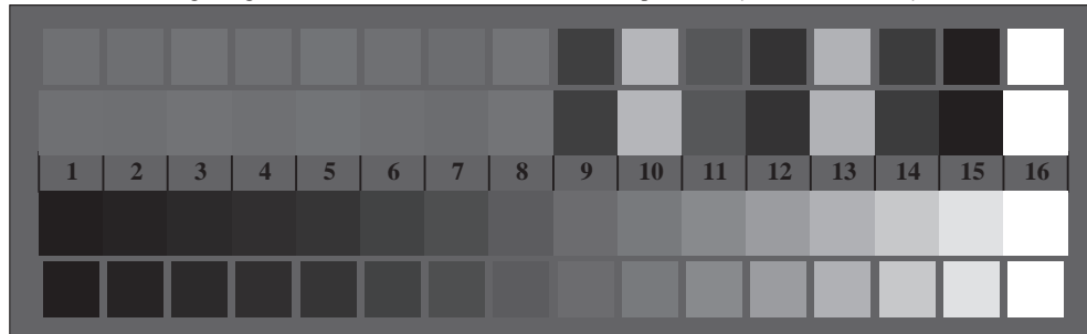
Picture B3: 14 CIE-test colours and 2 + 16 grey steps; Use of PS operator cmy0*/000n* setcmykcolor
