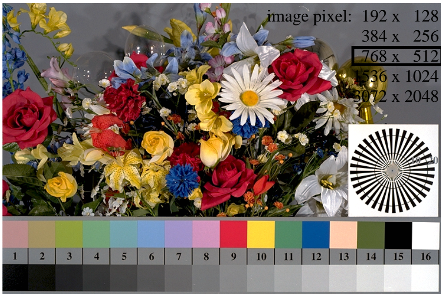
Picture D1: Flower motif, 14 CIE-test colours and 16 grey steps (nf); PS operators settransfer , 3 colorimage
