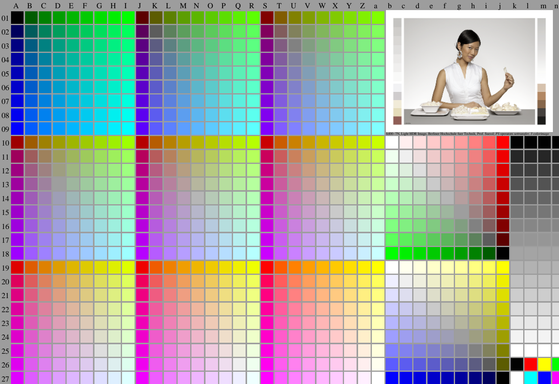
fel00-7N, Page 1/16, Test chart 2G with 40x27=1080 colours; digital equidistant 9 or 16 step colour scales; Colour data in column (A-n): rgb^* (A_n) , colorm = 1 , xchart = 4 , pchart = 0
