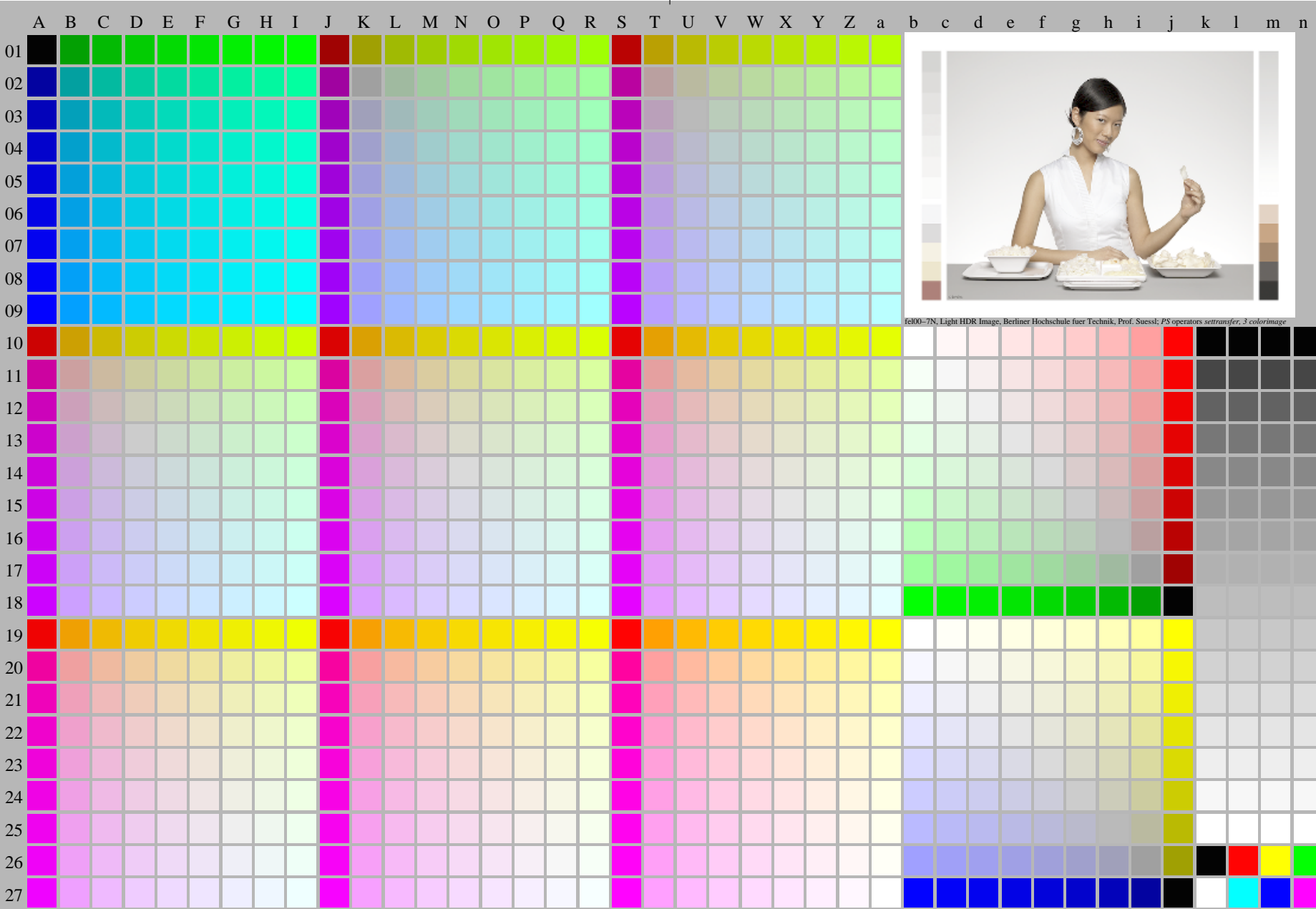
fel00-7N, Page 1/16, Test chart 2G with 40x27=1080 colours; digital equidistant 9 or 16 step colour scales; Colour data in column (A-n): rgb^* (A_n) , colorm = 1 , xchart = 7 , pchart = 0
