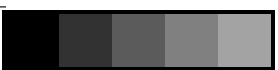
fek90-7N-132-2: 16 visual equidistant L^* -grey steps; PS operator: w^* w^* w^* setrgbcolor
