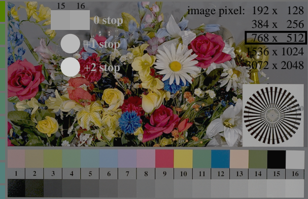
image pixel: 192 x 128 384 x 256 768 x 512 1536 x 1024 3072 x 2048 1 2 3 4 5 6 7 8 9 10 11 12 13 14 15 16 fek90-7N, Picture B1-136-0: Flower motif, 14 CIE-test colours and 2+16 grey steps (n); PS operators settransfer, 3 colorimage
