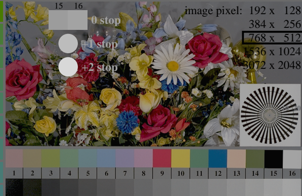
fek90-7N, Picture B1-135-0: Flower motif, 14 CIE-test colours and 2+16 grey steps (nd); PS operators settransfer, 3 colorimage
