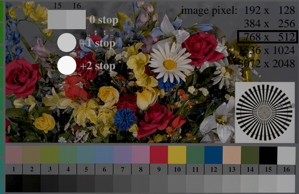
fek90-7N, Picture B1-131-0: Flower motif, 14 CIE-test colours and 2+16 grey steps (nd); PS operators settransfer, 3 colorimage
