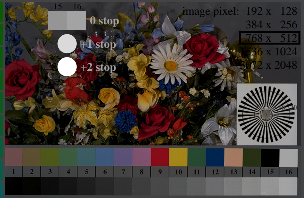
fek90-7N, Picture B1-130-3: Flower motif, 14 CIE-test colours and 2+16 grey steps (nd); PS operators settransfer, 3 colorimage
