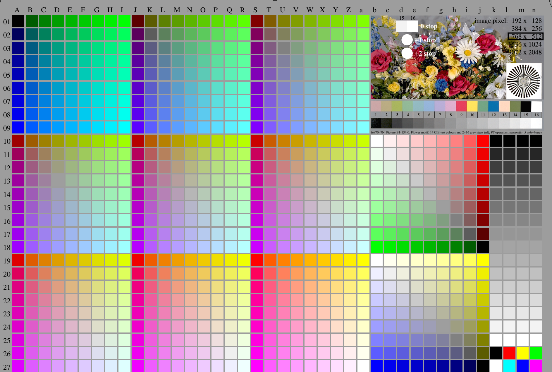
fek70-7N, Page 1/16, Test chart 2G with 40x27=1080 colours; digital equidistant 9 or 16 step colour scales; Colour data in column (A-n): rgb^*_d(A_n) , colorm = 1, xchart = 4, pchart = 0
