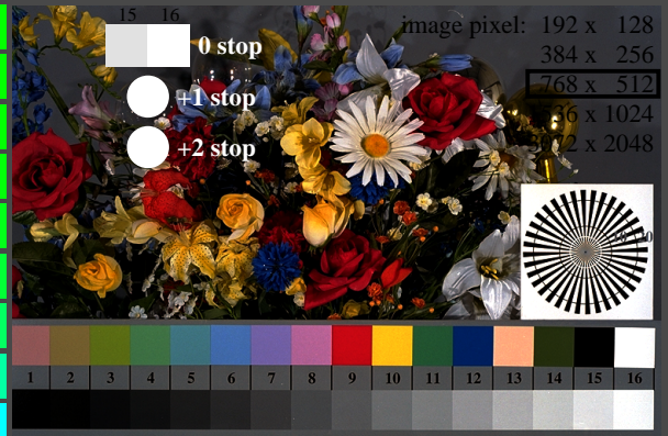
fek70-7N, Picture B1-130-6; Flower motif, 14 CIE-test colours and 2x 16 grey steps (nd); PS operators settransfer, 3 colorimage
