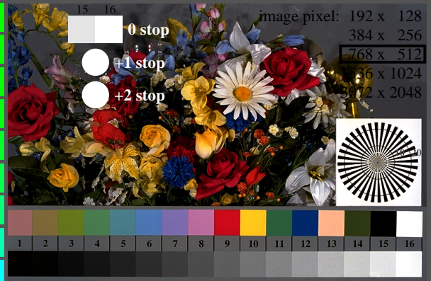
fek70-7N, Picture B1-130-5: Flower motif, 14 CIE-test colours and 2+16 grey steps (nd); PS operators settransfer, 3 colorimage
