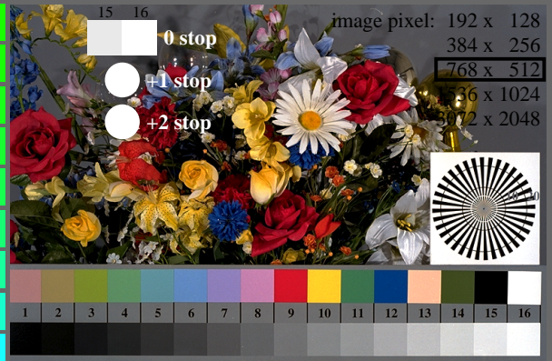
fek70-7N, Picture B1-130-3: Flower motif, 14 CIE-test colours and 2+16 grey steps (nd); PS operators settransfer, 3 colorimage
