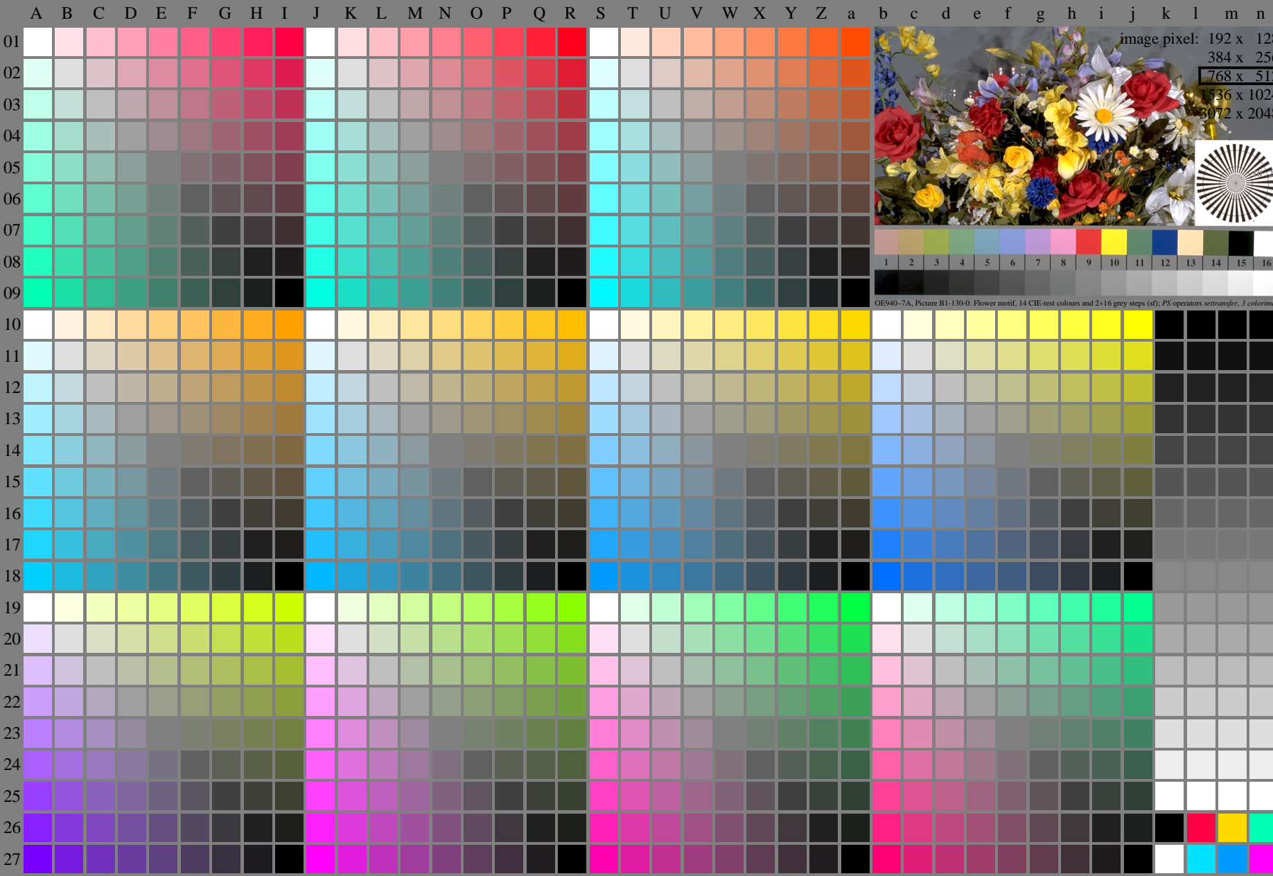
fei90-7N, Page 1/16, Test chart 2E with 40x27=1080 colours; digital equidistant 9 or 16 step colour scales; Colour data in column (A-n): rgb^*_{de} (A_n), colorm = 1, xchart = 0, pchart = 0
