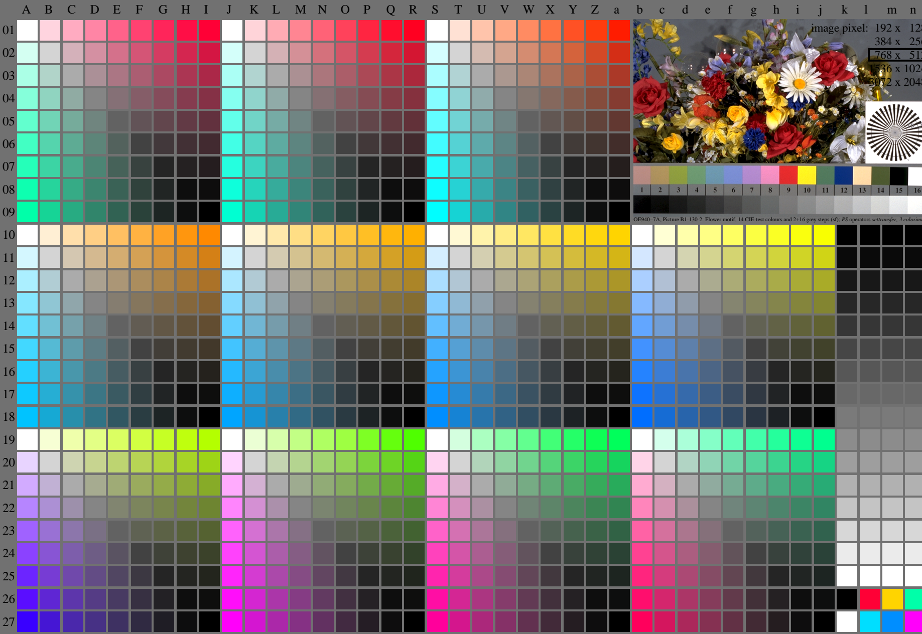
fei90-7N, Page 1/16, Test chart 2E with 40x27=1080 colours; digital equidistant 9 or 16 step colour scales; Colour data in column (A-n): rgb^*_{A_n} , colorm = 1 , xchart = 16 , pchart = 0
