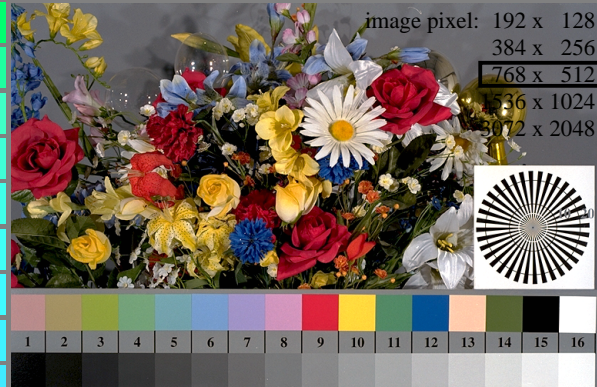
fei80-7N, Picture B1-130-0: Flower motif, 14 CIE-test colours and 2+16 grey steps (n); PS operators settransfer, 3 colorimage
