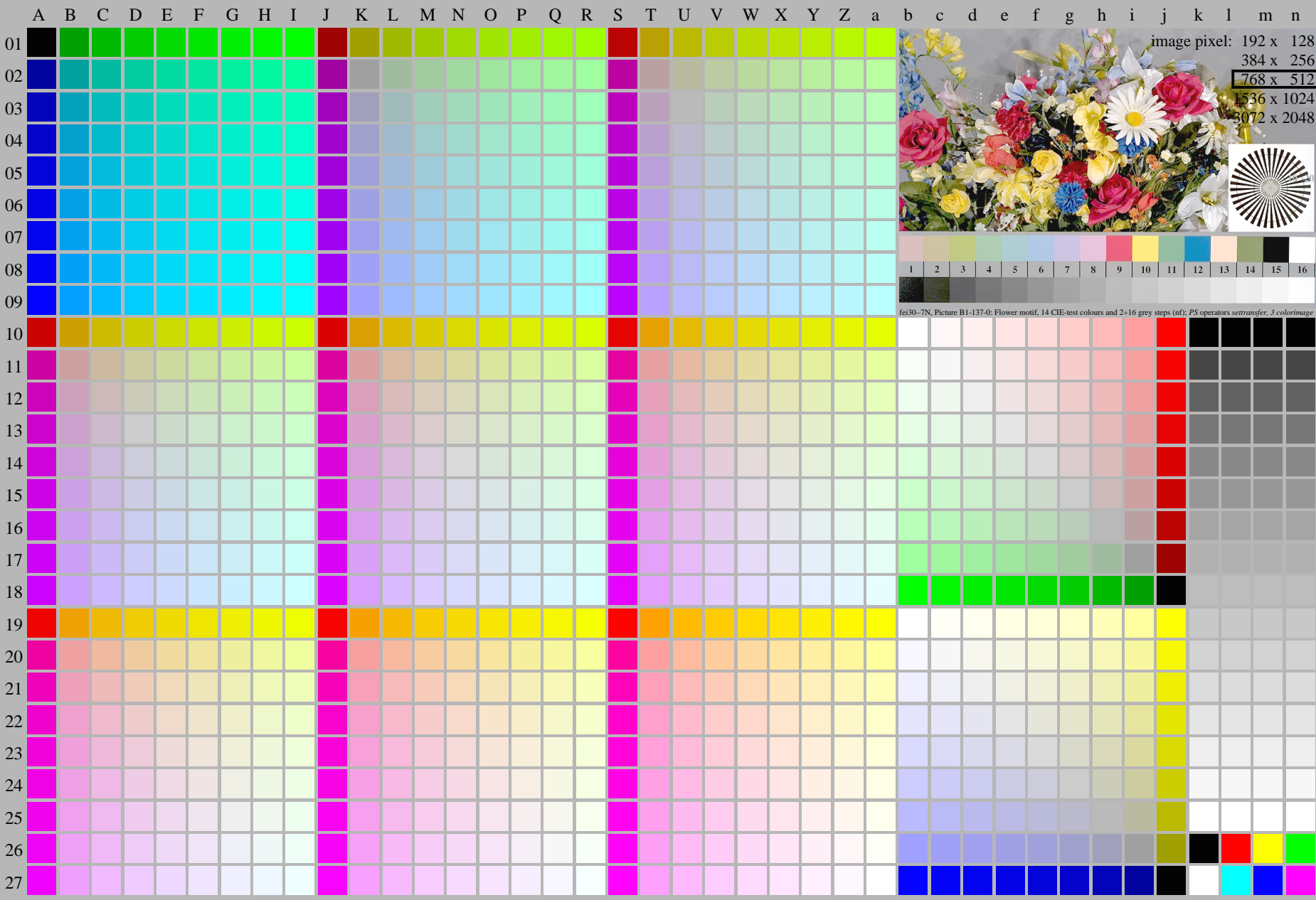
fei30-7N, Page 1/16, Test chart 2G with 40x27=1080 colours; digital equidistant 9 or 16 step colour scales; Colour data in column (A-n): rgb^* (A_n) , colorm = 1 , xchart = 7 , pchart = 0
