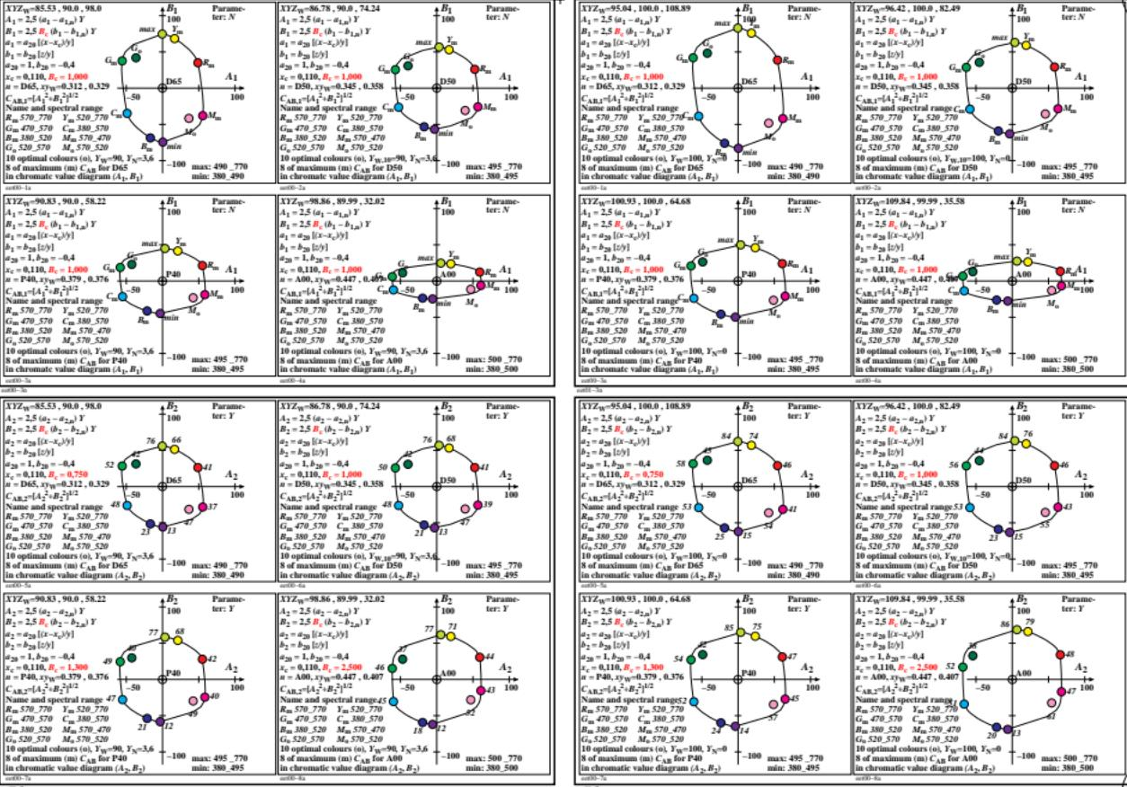
TUB-test chart ee0; Ostwald optimal colours,  $Y_w=90 \pm 100$ , D65, D50, P40, A00, CIE-02-degree Antagonistic hue circle, approximately constant chromatic value CAB,2 for contrast  $C=288:1$
