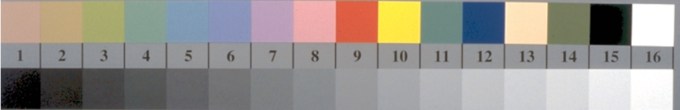
RE970-7, Picture B1-131-0: Flower motif, 14 CIE-test colours and 2 + 16 grey steps (sf6); PS operators settransfer , 4 colorimage
