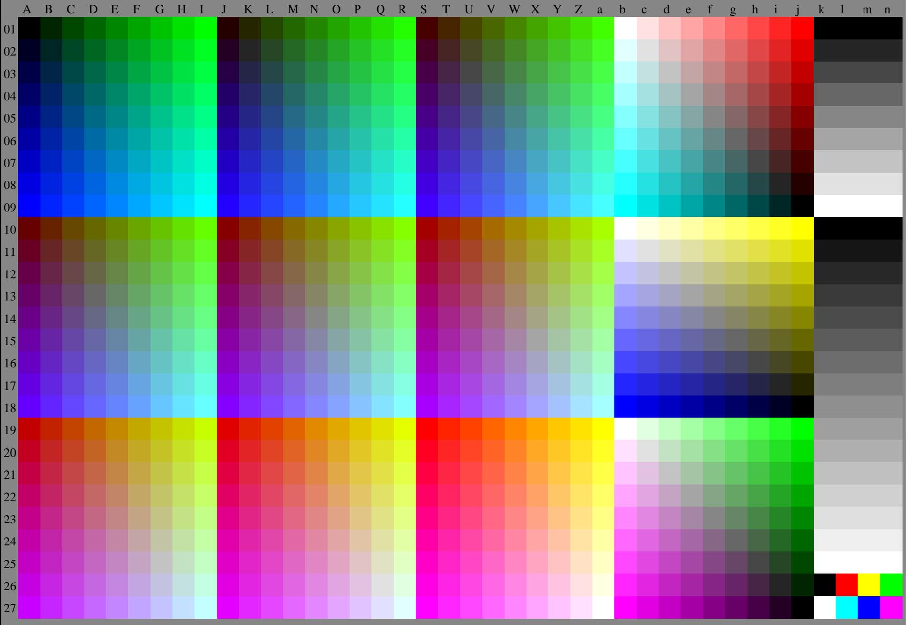
Test chart G with 40x27=1080 colours; digital equidistant 9 or 16 step colour scales; Colour data in column (A-n):  $rgb(A_n), 3D=0$
