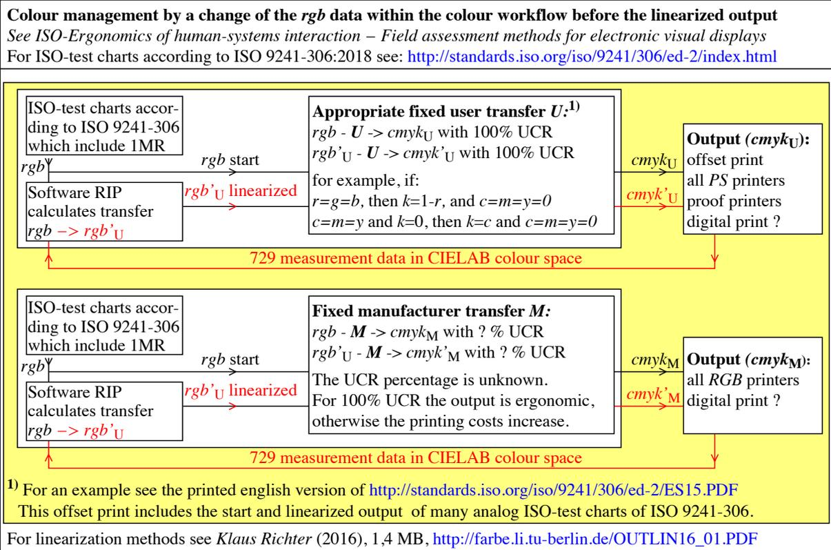
**Figure 8: Transfer of  $rgb_d$  to  $cmyk_d$  colour values for offset and printer output**
