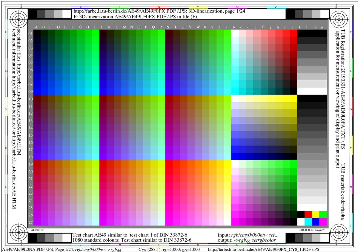
**Figure 4: TUB-test chart AE49 with relative ISO gamma  $g_p=1,000$  (ISO-contrast step  $C_{YP8}$ ), use the ISO file <http://standards.iso.org/iso/9241/306/ed-2/AE49/AE49F0PX.PDF>. Figure 4 contains 729 (=9x9x9) colours in the rows 01 to 27 and the columns A to a. These 729  $rgb_d$ -colour values are used to steer the colour output and input. Within the Columns  $b$  to  $n$  colours that are particularly suitable for visual assessments.**
