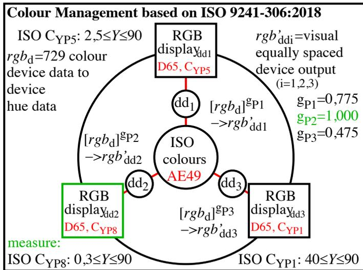
**Figure 5: Colour output of the ISO-test chart AE49 for three ISO-contrast steps**
