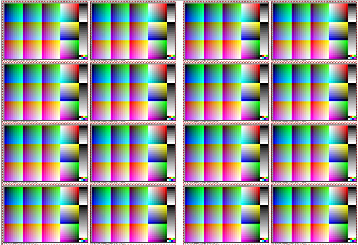
**Figure 13: 16 identical ISO-test charts AE49 with the relative ISO gamma  $g_p = 0,775$  (ISO-contrast step  $C_{YP5}$ ), see <http://farbe.li.tu-berlin.de/AEW7/AEW70-7N.PDF>.**
