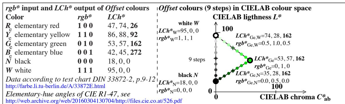
**Figure 3: Elementary colours with  $rgb^*$  and CIELAB- $LCh^*$  colour values**
