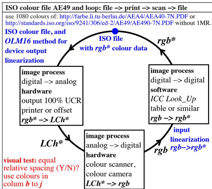
**Figure 2: Colour loop: ISO-colour file – print - scan and back to the ISO-colour file**
