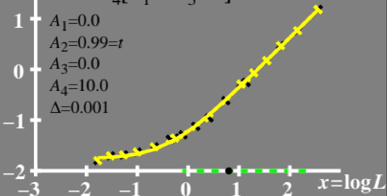
$\log(L/\Delta L)$  luminance contrast sensitivity threshold •  $L_g = 6.3 \text{ cd/m}^2$
