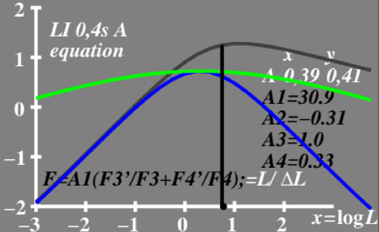
$\log L/\Delta L$  luminance contrast sensitivity threshold •  $L_g=60\text{cd/m}^2$
