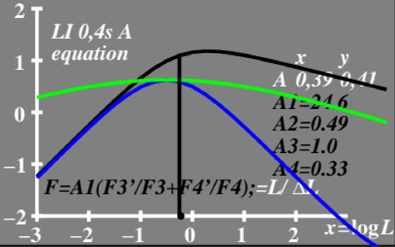
$\log L/\Delta L$  luminance contrast sensitivity threshold •  $L_g=6\text{cd}/\text{m}^2$
