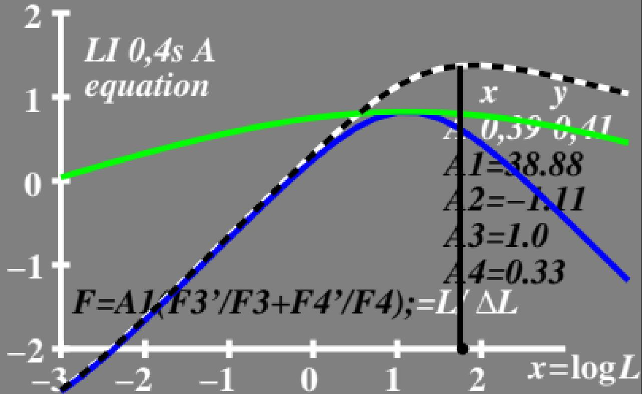
$\log L/\Delta L$  luminance contrast sensitivity threshold •  $L_g=600\text{cd/m}^2$
