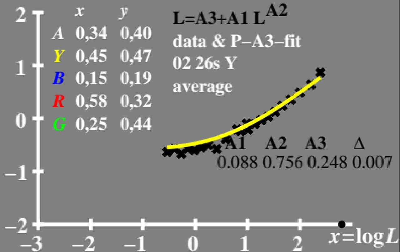
log  $\Delta L$  luminance difference threshold  $\bullet L_g=63\text{cd/m}^2$
