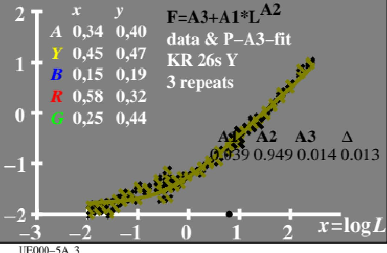
$\log L/\Delta L$  luminance contrast sensitivity threshold •  $L_g = 630 \text{ cd/m}^2$
