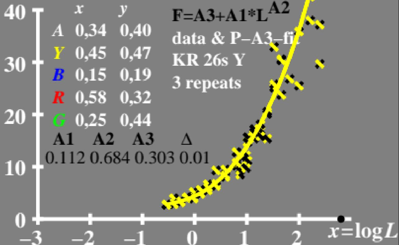
$L/\Delta L$  luminance contrast sensitivity threshold  $L_g = 63 \text{ cd/m}^2$
