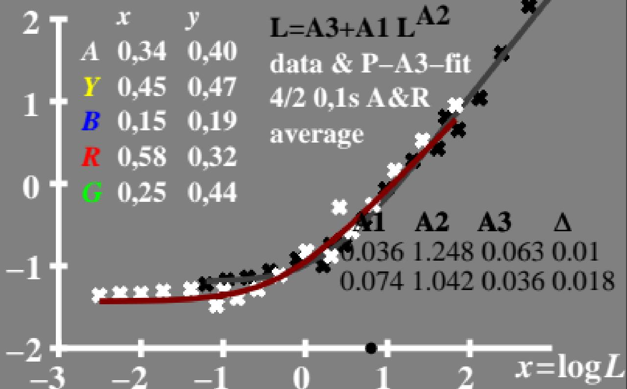
$\log L/\Delta L$  luminance contrast sensitivity threshold •  $L_g=630\text{cd/m}^2$
