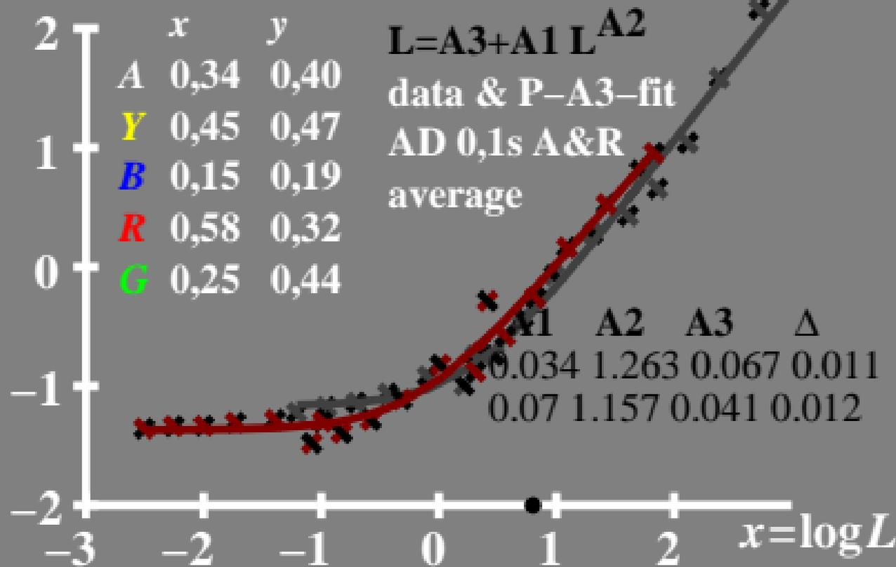
$\log L/\Delta L$  luminance contrast sensitivity threshold  $\bullet L_g=630\text{cd/m}^2$
