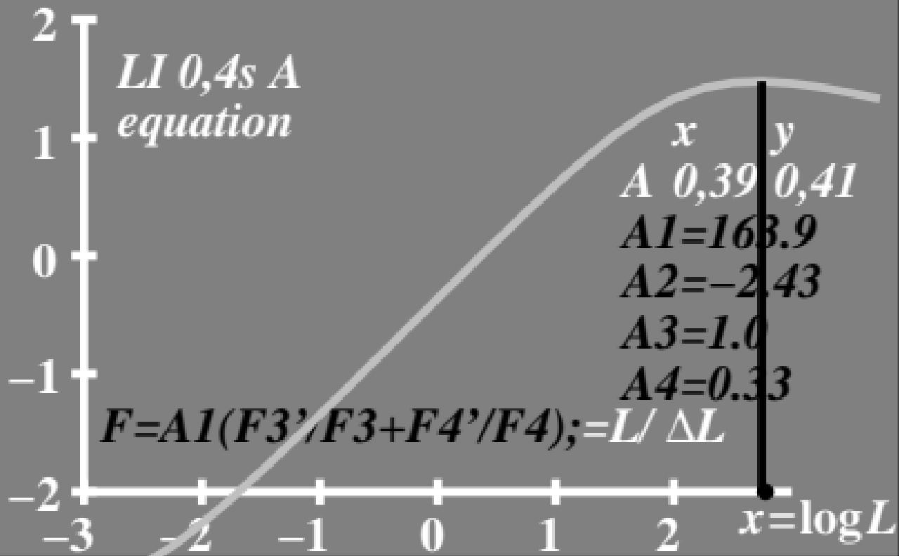
$\log L/\Delta L$  luminance contrast sensitivity threshold •  $L_g=6000\text{cd/m}^2$
