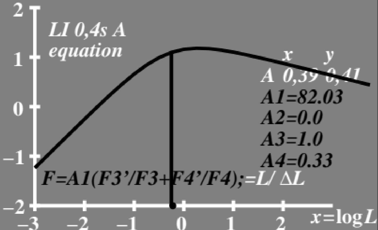
$\log L/\Delta L$  luminance contrast sensitivity threshold •  $L_g=6\text{cd}/\text{m}^2$
