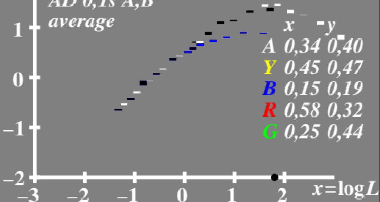
$\log L/\Delta L$  luminance contrast sensitivity threshold •  $L_g=6,3\text{cd}/\text{m}^2$
