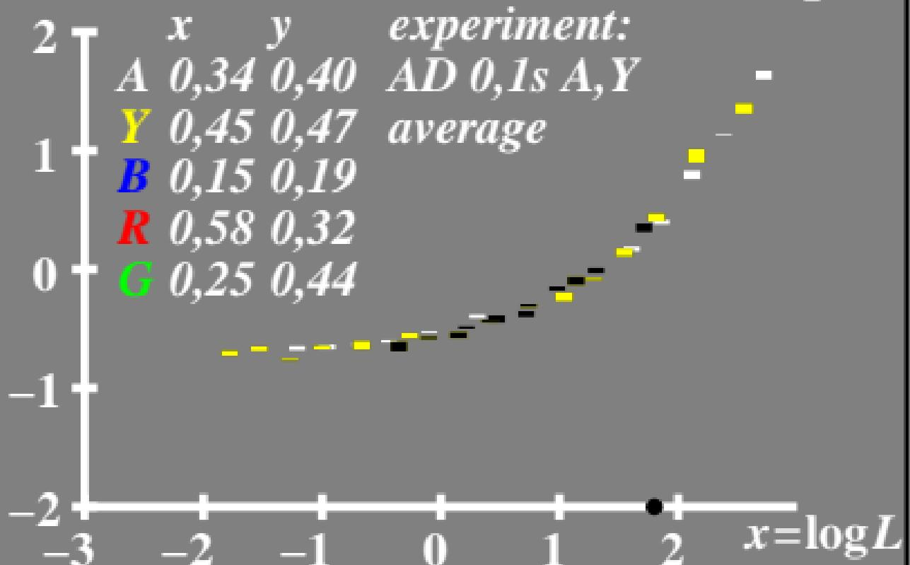
$\log \Delta L$  luminance difference threshold •  $L_g=6,3\text{cd}/\text{m}^2$
