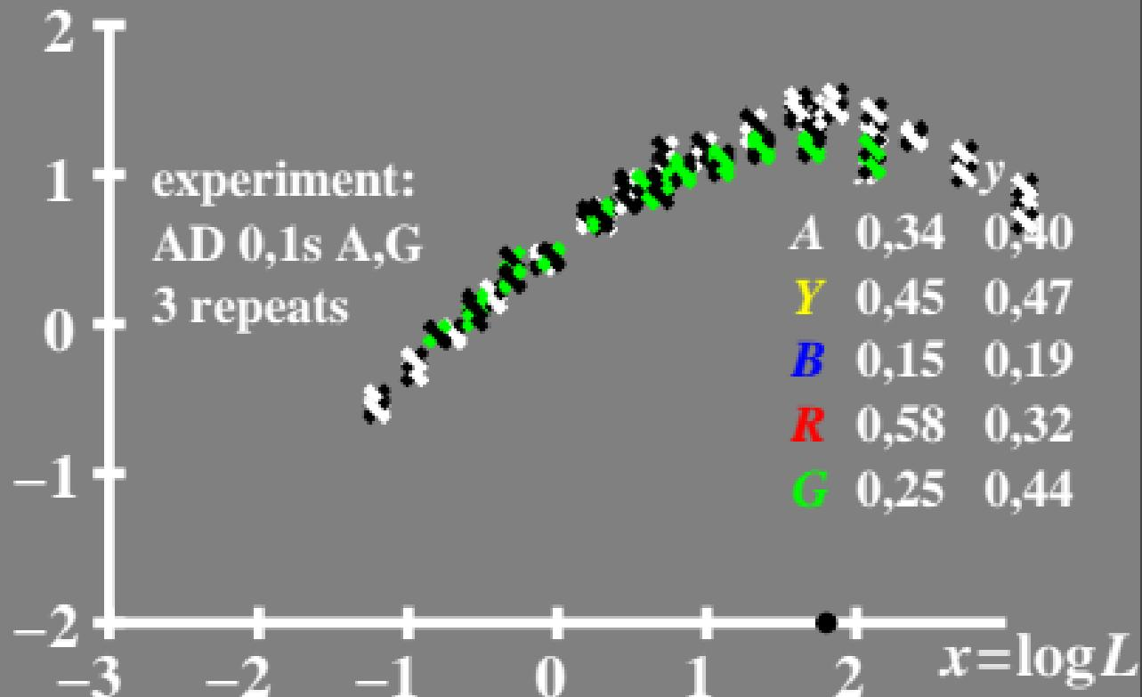
$\log L/\Delta L$  luminance contrast sensitivity threshold •  $L_g=6,3\text{cd/m}^2$
