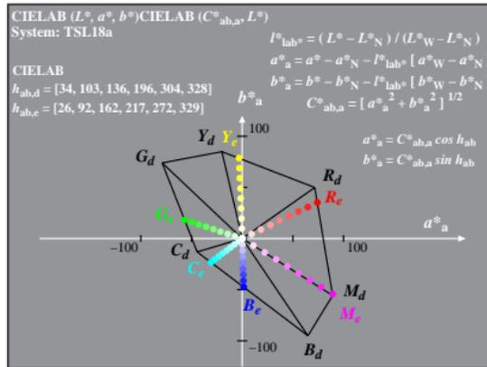
gráfico TUB-SS27; 4 device systems and CIE elementary hue data in CIELAB chroma diagram ( $a^*$ ,  $b^*$ )
