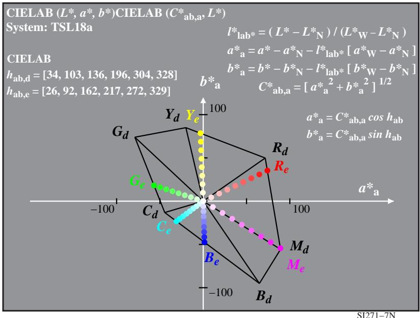
grafico TUB-SI27; 4 device systems and CIE elementary hue data in CIELAB chroma diagram ( $a^*, b^*$ )
