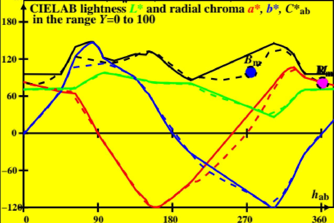
CIE data for antichromatic optimal colours of maximum chromatic value for P40,  $Y_w=100$ ,  $Y_m=520$  770,  $B_m=380$  520
