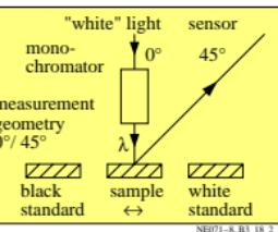
TUB-test chart NE07; Richter: Computer graphics, colorimetry
