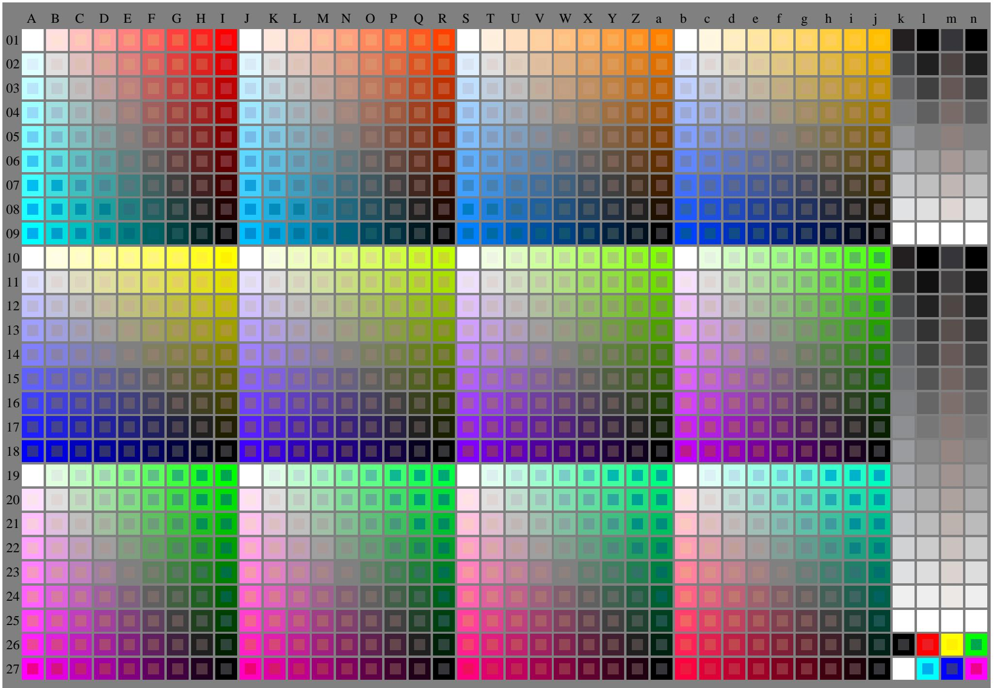
LE770-7N, 1/5, Test chart O with 40x27=1080 colours; digital equidistant 9 or 16 step colour scales; Colour data in column (A-n): **rgb + cmy0 (A\_j + k26\_n27), 000n (k), w (l), mnn0 (m), www (n), colorm = 0, separation = A**
